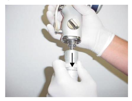
• Slide quick-disconnect outer-shell in direction shown to secure hose to the Woodpecker.
