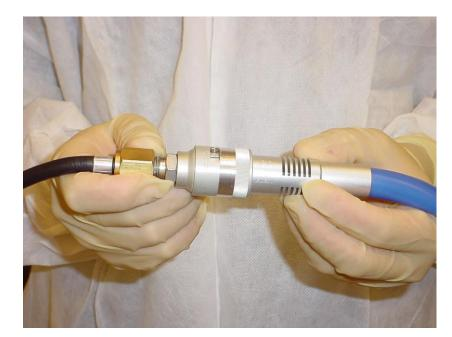
• IMT AG recommends starting at 100 PSI (7 bar). Effective pressure range is 87 to 120 PSI (6-8 bar).
