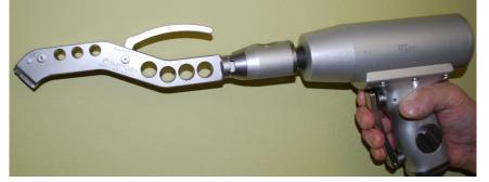
• Insert broach into broach adapter. Lock into place.
